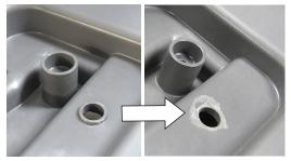
If replacing the operator presence pedal switch, position the green wire as shown and secure it with tape to prevent wire damage.
